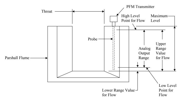
Determine the Maximum Level. This is the highest point that can possibly be measured. This is usually, but not always, the same as the height of the throat. Fill in the value below.
